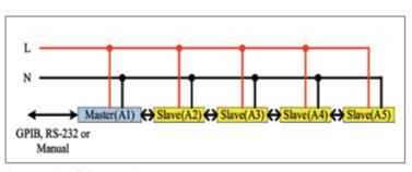
Figure 10: Parallel connection
