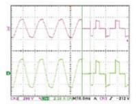
Figure 7 : Transfer time for Off-Line UPS
