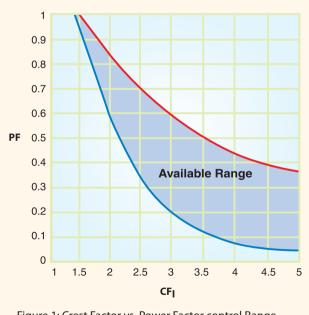
Figure 1: Crest Factor vs. Power Factor control Range
