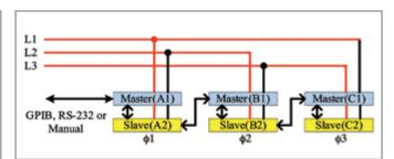
Figure 12: Parallel/3-Phase Delta connection
