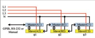
figure 11: Parallel/3-Phase Y connection
